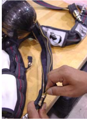
Installing hose cover
